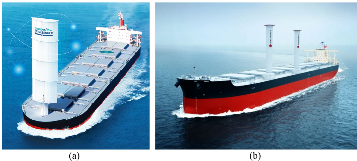
Fig. 1 Wind assisted ships equipped with rigid wind sails [6], and rotor sails [7]
