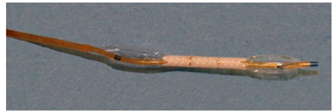
Fig. 2 ▲ A PLLA/P4HB stent mounted on a PTA balloon catheter and predilated extracorporeally with 1 bar
