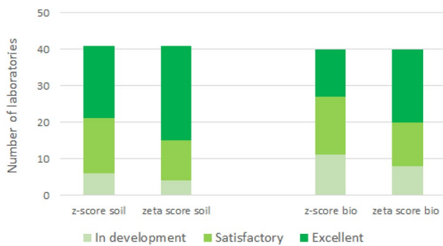
Fig. 7 Number of NAA laboratories participating in the 2018 round, categorized to their level of performance on basis of z -score and zeta score. ‘Bio’ refers to the analysis of plant and animal tissue. One laboratory only analysed the soil sample, and not the bio sample
