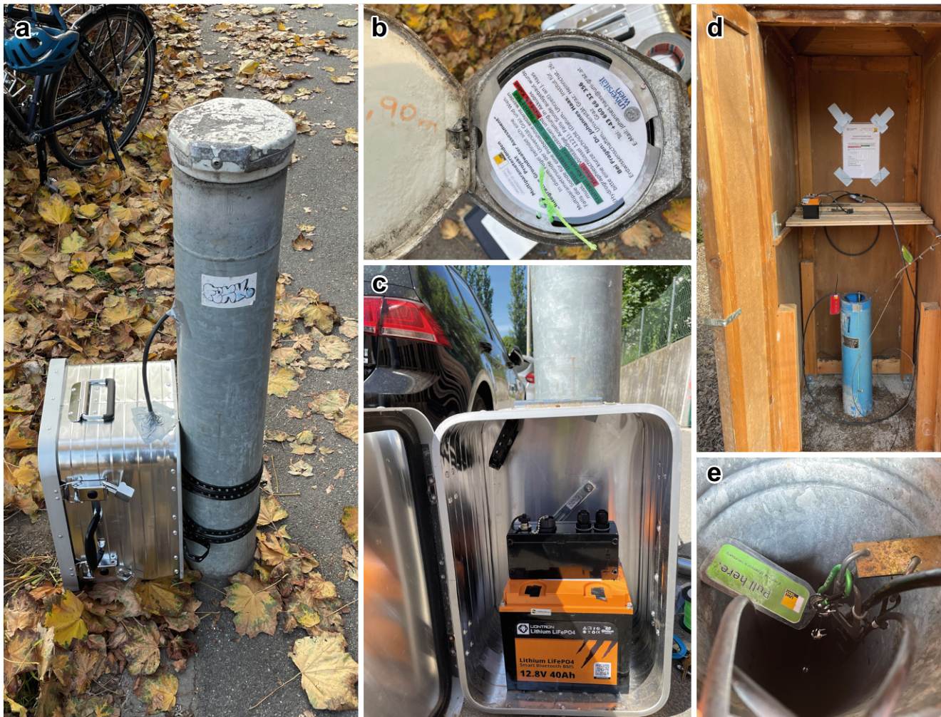
Fig. 2 Setups of the spectrolysers at the well sites; a Outside view of a well head with battery box; b Removal instructions placed into the well head; c Inside of the battery box, attached to well head; pictured is a large, 40Ah battery with a connection box for the brushing system and additional space in the box for cables or an even larger 55 Ah battery. The Battery box is approx. 45 × 30 × 28 cm in size; d Removal instructions taped to the wall of the well hut, with red and green “do not pull!”/“pull here” markers on the cables; e “pull here” marker and a green carabiner needed to attach the spectrolyser to a non-standard attachment point inside a well head
