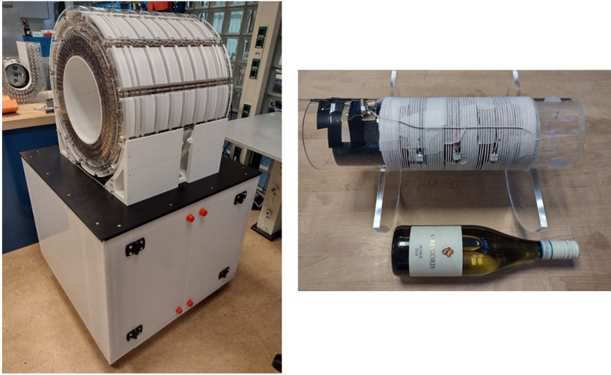
Fig. 1 (left) Photograph of the 46 mT portable Halbach-based MRI system. Electronics are located within the cabinet below the scanner. Shim trays are placed around the outside of the magnet. (right) Photograph of the segmented solenoid transmit/receive coil next to the wine bottle. Plastic supports ensure that the bottle is in the center of the magnet
