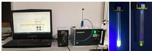
Fig. 2 Experimental setup. Left image: MR benchtop system with laptop, research control unit, and magnet with removable ^{19}\text{F} coil. Middle image: NMR tube containing 3-Fluoro-DL-tyrosine/riboflavin 5'-monophosphate. The glass fiber is centrally positioned, and the tip of the glass fiber is located approximately in the middle of the sample volume. The sample is illuminated with high intensity light. Right image: The stronger illumination below the glass fiber tip and the reduced illumination in the upper half of the sample volume where light exits laterally from the glass fiber is more clearly seen under low intensity conditions
