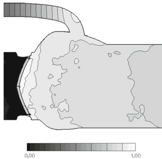
Fig. 13 Pressure distribution in the D – D plane after valve closure for the three sinuses prosthesis: \frac{p - p_{ref}}{\rho u_{ref}^2} , where p_{ref} is the left ventricular pressure
