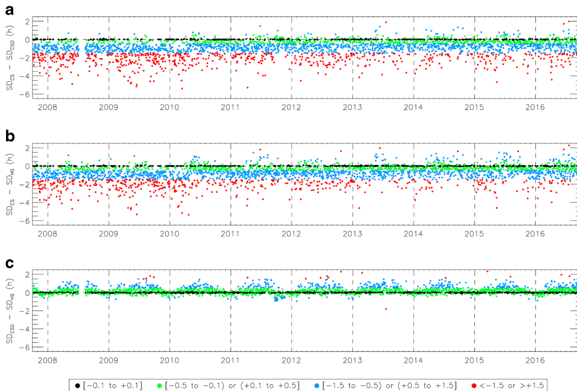
Fig. 2 Differences in daily sunshine duration (SD) totals among instrument pairs. a CS/CSD. b CS/HS. c CSD/HS, with color-coding following the Urban and Zając (2016) classification scheme
