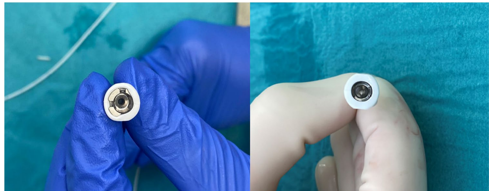
Fig. 5 Curled up silicone layer surrounding the sutureless pump connector (left) and normal silicone layer surrounding the sutureless pump connector (right)
