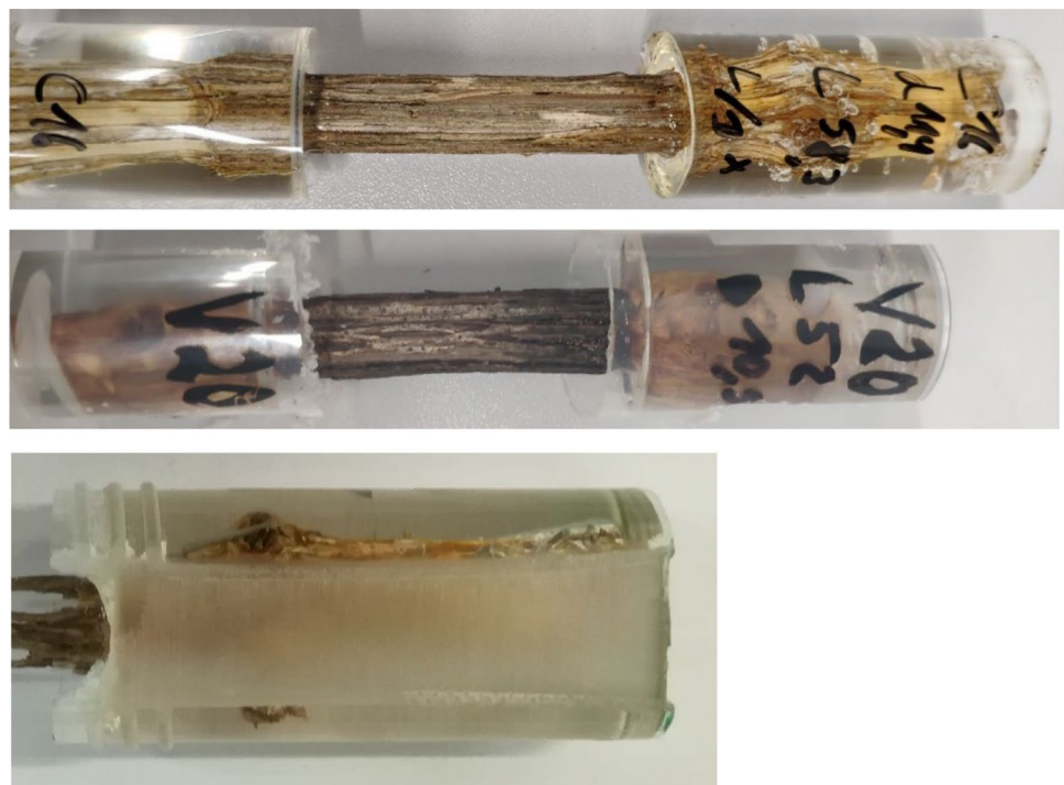
Fig. 2 Characteristic specimens of both species. Top: C16 specimen, diameter 11.6 mm. Middle: V20, Vitis vinifera specimen, diameter 10.9 mm. Bottom: sanded surface for fixation
