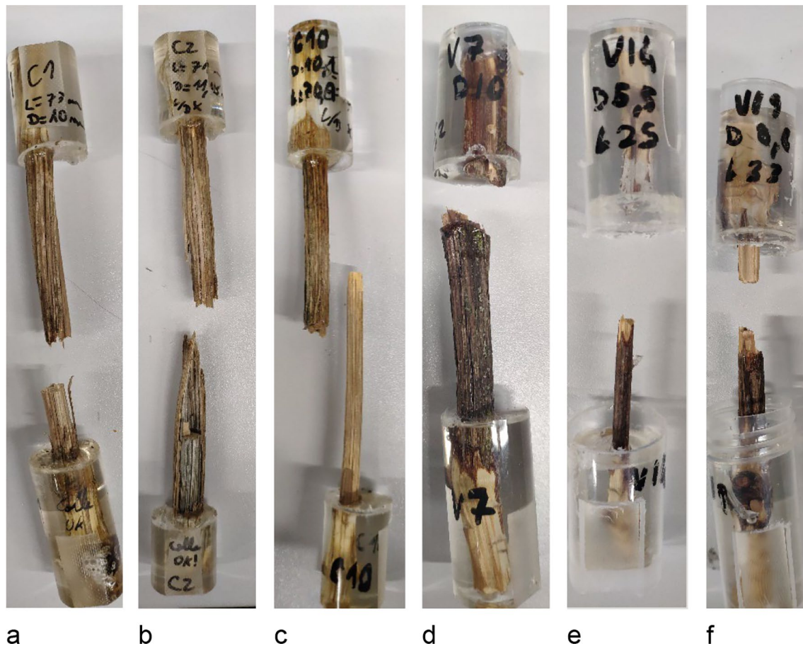
Fig. 11 Typical examples of failure modes of Clematis vitalba (C) and Vitis vinifera (V) specimens. a C1, b C2, c C10, d V7, e V14, f V19
