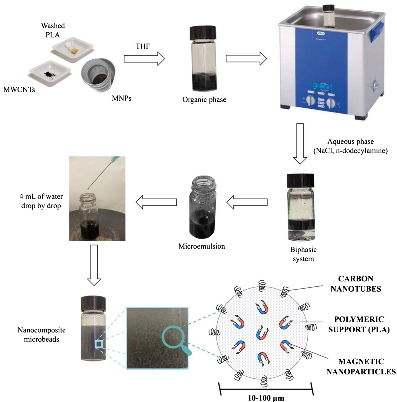
Fig. 1 Representation of the synthetic strategy for the realization of mPLA@MWCNTs(5) nanocomposites and schematic image of the final material structure
