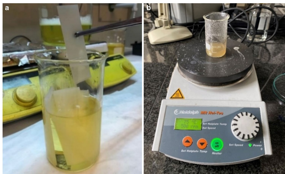
Fig. 3 Preparation of the LOC substrates: (a) multi-jet 3D printed substrates prior to heating in oil-bath, (b) preparation of polymer solution for hydrogel matrices
