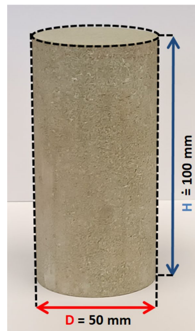
Fig. 3 A sample of the Brenna sandstone prepared for mechanical testing
