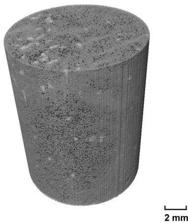
Fig. 6 X-ray tomography of specimen, S4 saturated with Krypton (Lighter gray represents the higher concentration of Krypton)
