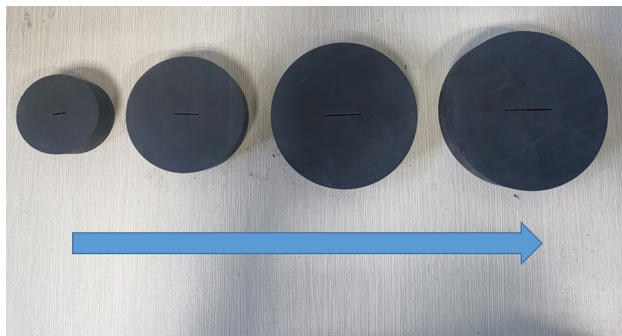
Fig. 3 The CSTBD specimens manufactured in four different sizes
