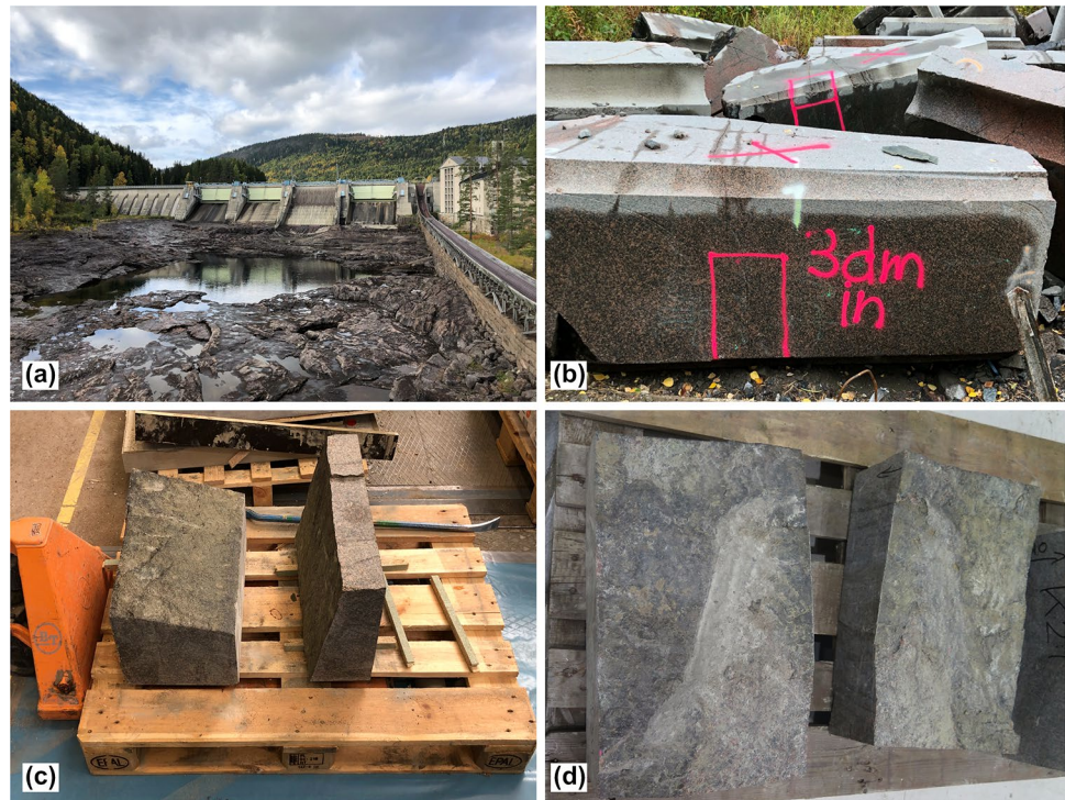
Fig. 3 a Concrete dam at Krångede; b large rock blocks obtained by wire-cutting and lifted up during the excavation of the vertical shafts (the marks in magenta colour indicate the dimensions for laboratory sample cutting); c rock joint sample K1 before encapsulation in the specimen holder; d rock joint sample K2 before encapsulation in the specimen holder
