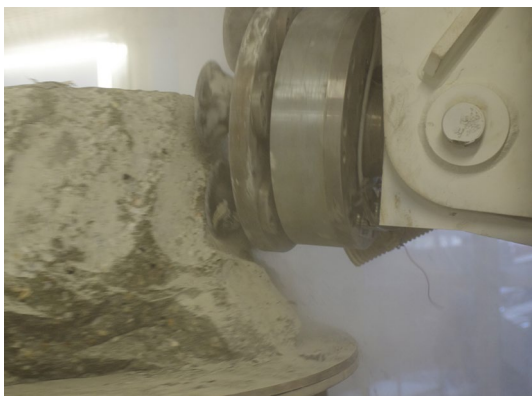
Fig. 27 Laboratory tests with the single disc plate
