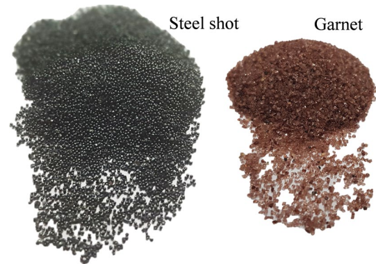
Fig. 1 Abrasives for experiment: steel shot and garnet
