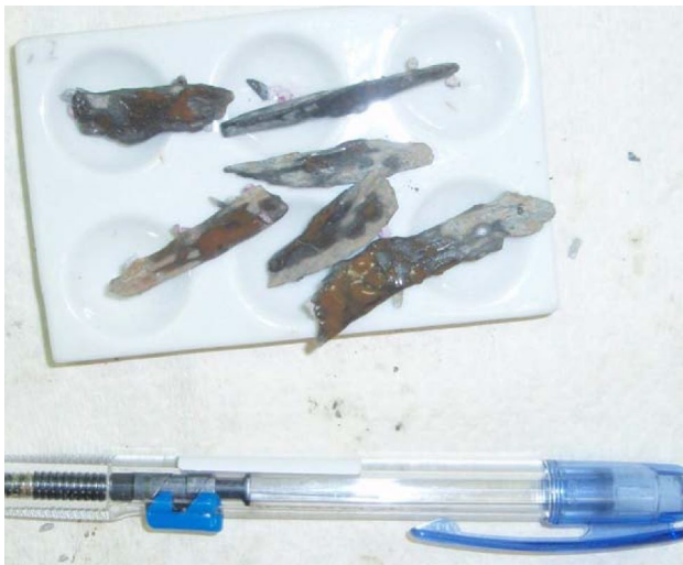
Fig. 15 Splintery cuttings from breakouts in a thick shale section in the existing vertical well
