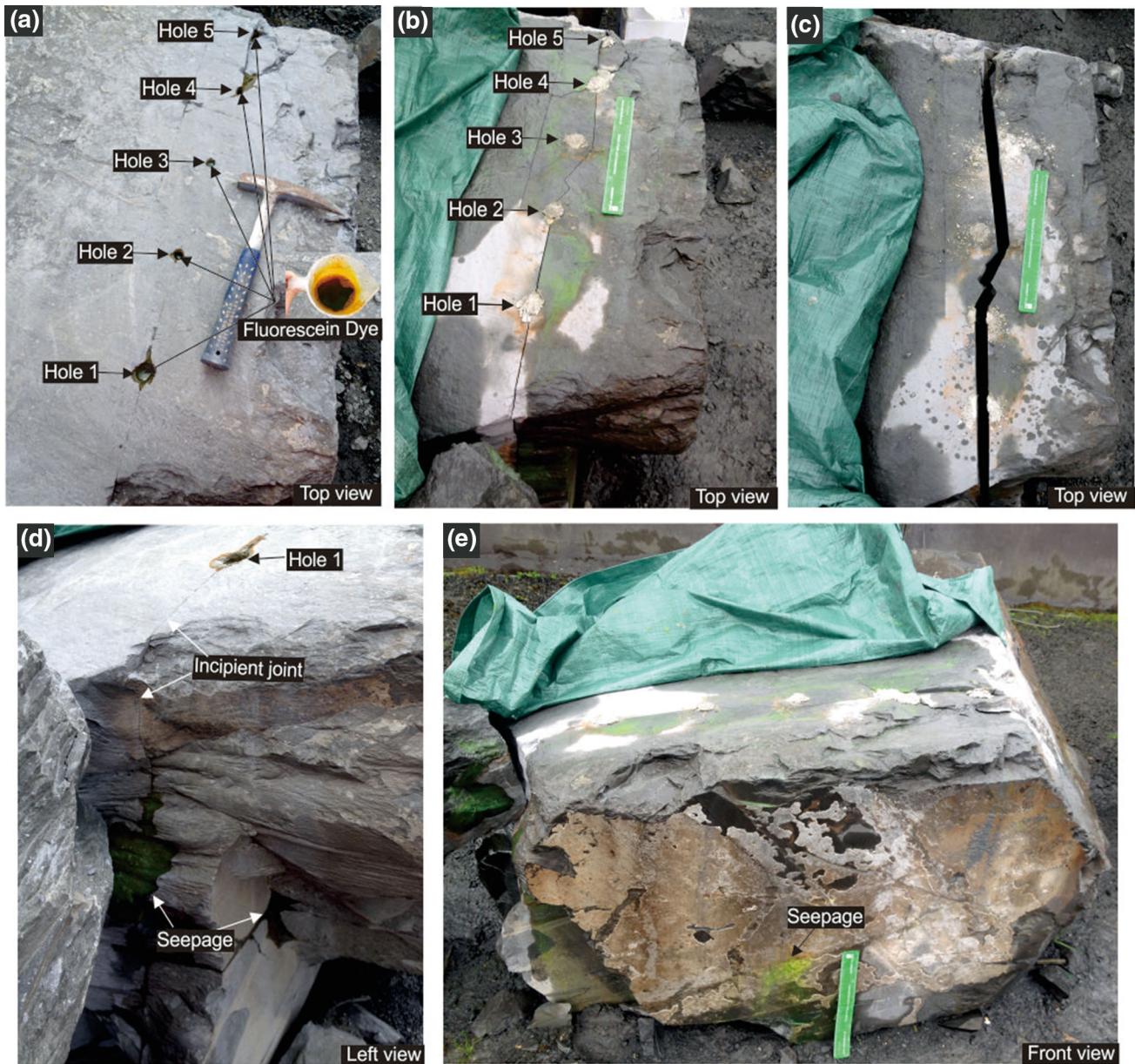
Fig. 16 FERM testing along incipient joint ① from the Horton Formation Siltstone block. a Fluorescein dye ( C_{20}H_{12}O_5 ) was poured into the pre-drilled holes prior to the forensic splitting. b Chemical splitter was injected and one fracture with an aperture of about 2 mm
