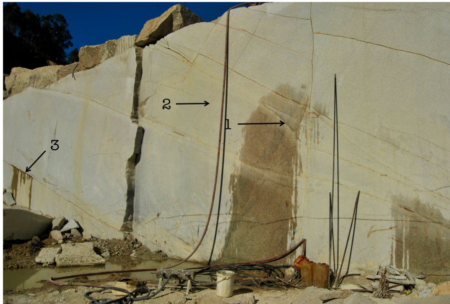
Fig. 2 Face cut by diamond wire saw in dimension stone quarry near Tui, Galicia, Spain. Sets of joints can be seen as linear traces stained with iron oxides, cutting the granite. These joints were evidently formed from brittle fracture propagation at a late stage during cooling/emplacement of the granite as can be interpreted from cross-cutting relationships and the geometrical association of some joints with mineral differentiation (as at 1 in an area washed off with water). Note that some of the joints are poorly defined and terminate (as
