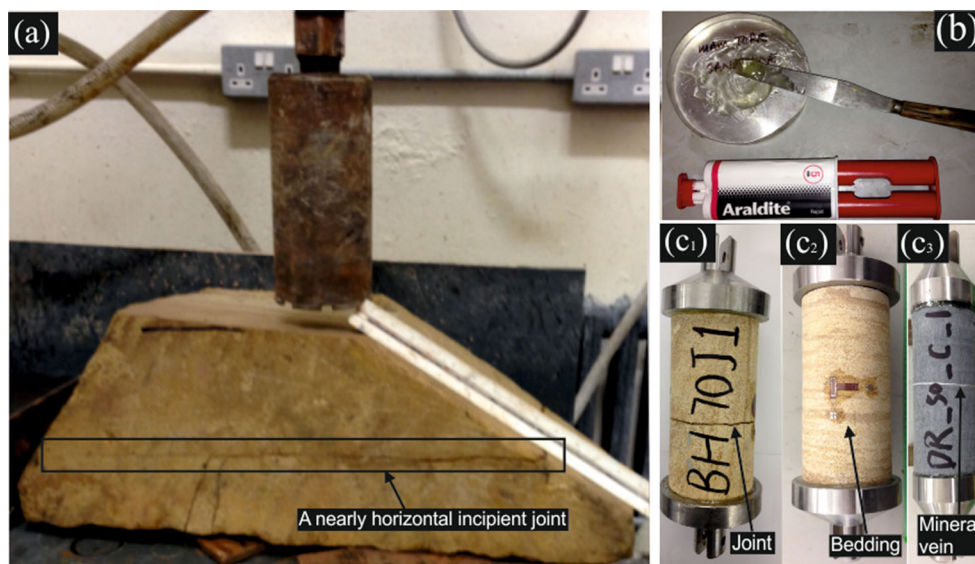
Fig. 4 Sample preparation. a Sandstone cores drilled perpendicular to an incipient joint within a large size sandstone block. b Araldite was used to cement metal caps to sample ends. Samples containing a single visible joint (c 1 ), bedding planes (c 2 ) and a mineral vein (c 3 )
