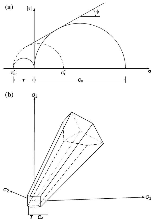
**Fig. 3** Tension cut-offs for the modified Mohr-Coulomb failure criterion: **a** failure envelope in the Mohr diagram; **b** representation in principal stress space
