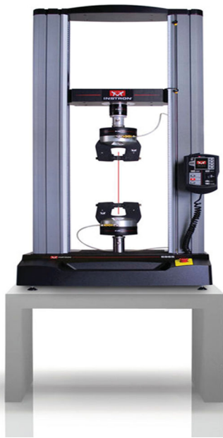
Fig. 1 Computerized testing machine Instron 5965L1684 was used in biomechanical testing of bone cement and bisphosphonate-enriched bone cement
