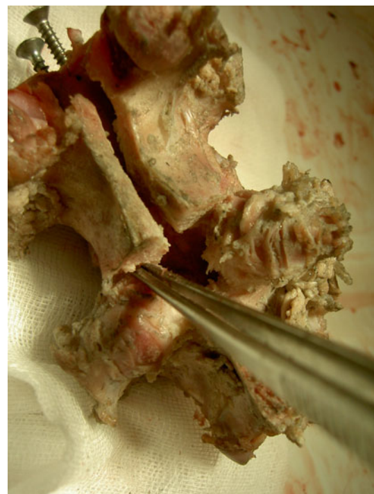
Fig. 4 The tweezers show a pars interarticularis fracture after testing a laminectomy and partial facetectomy segment
