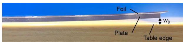
Fig. 16 Side view of a sample fabricated by friction embossing lying on a table
