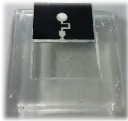
Fig. 2 Vinyl film master mold with geometry of microthruster design and replicated PDMS soft mold
