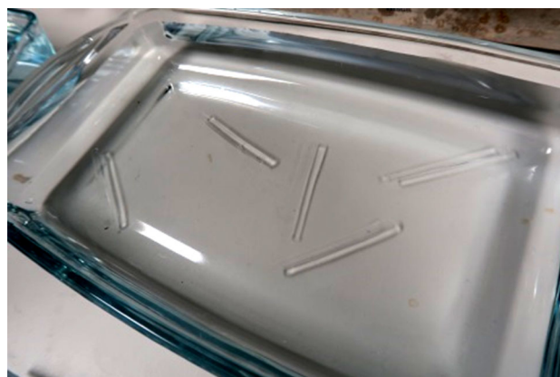
Fig. 5 Photo of swelling test setup with glass container filled with aqueous solutions with five PDMS strips of the same mixing ratio submerged
