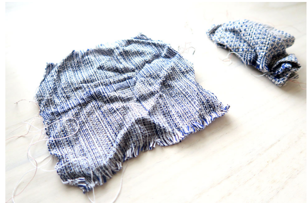
Fig. 24 Photo of e-textile samples after washing showing the sample stretched out (left) and sample deformed shape after washing cycle (right)
