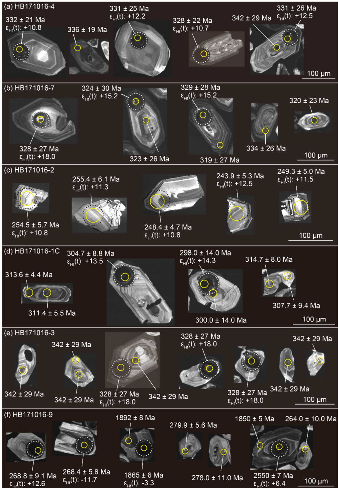
Fig. 6 CL images of the studied zircon grains from the Unazuki Belt. The U–Pb dating spots and Lu–Hf analytical spots are shown by solid and dashed circles, respectively. The dates with 2\sigma error and \epsilon_{\text{Hf}}(t) values are shown for each spot
