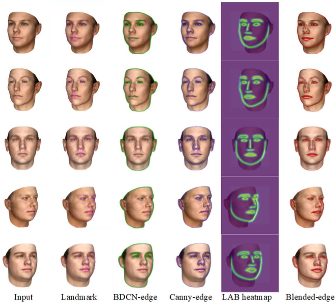
Fig. 6 Edge features and 3D face reconstructions for images from the synthetic dataset. From the left to right: inputs, landmarks, BDCN edges, hard Canny edges, LAB heatmaps, and hard-blended edges
