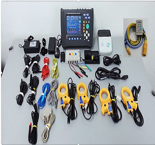
Fig. 14 The utilized power analyzer (model HIOKI-3196 with the program of HIOKI-9624-50 “PQA-Hiview PRO”)
