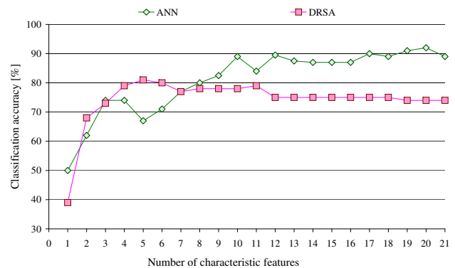
Fig. 10 Pruning of inputs for ANN classifier compared to pruning of rules from all rules on examples decision algorithm induced for the complete set of attributes, with dimensionality reduction executed while following DRSA Ranking
