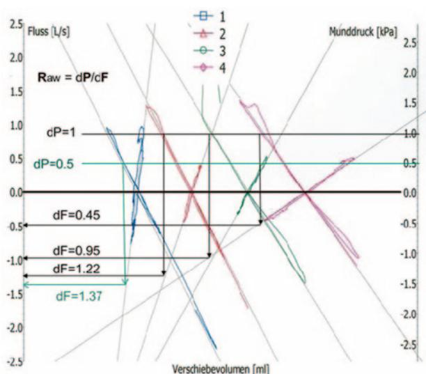
Not only do flow-volume-loops (unit=1/time) turn clockwise with external resistances added, but also does the slope  $dP/dV \approx 1/ITGV$  decrease indicating a gain in FRC.  $Raw (dP/dF)$  rises with flow limitation. Thus the specific resistance  $Raw \times ITGV = time$  increases even more meaning that filling and emptying of the lungs takes longer.
