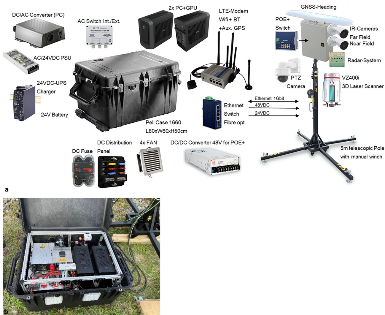
Fig. 2 a Illustration of a sensor station with its sensor head. b A closer look inside the protective case
