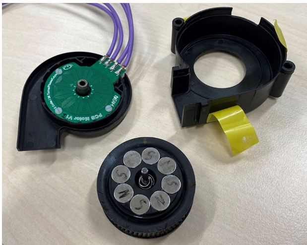
Fig. 6 Base plate with PCB, Rotor 2 and fan housing (configuration 4)
