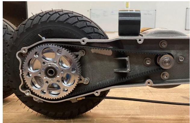
Fig. 2: Previous belt wheel mounted in the motor unit
