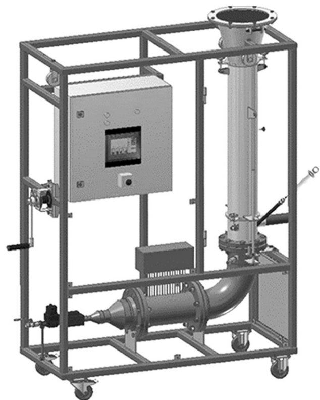
Fig. 2: 3D illustration of the triboelectrostatic charging unit [8]
