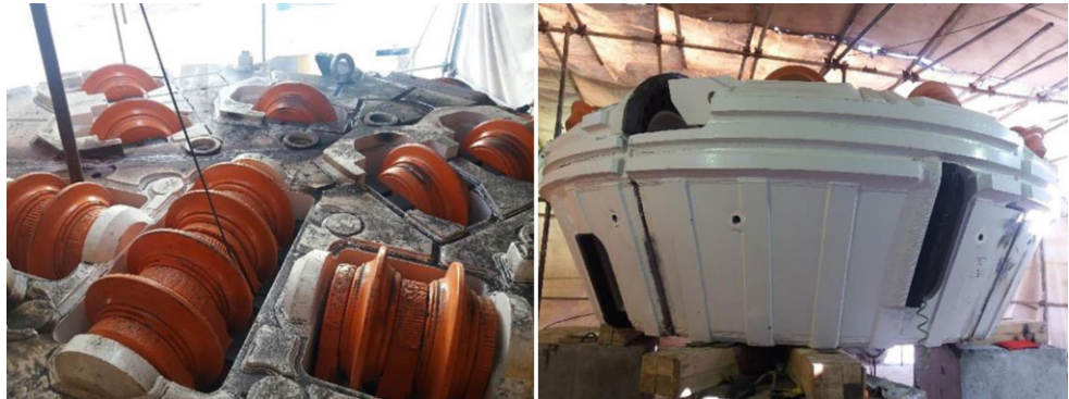
Fig. 5: The new cutterhead of TBM S323 to be applied on the northern lot of the Kerman tunnel
