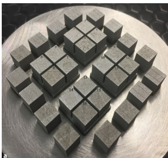
Fig. 4: a W blocks; b Density measured with Archimedes' method as function of hatch distance ( h_d ) at different scan speed ( v )
