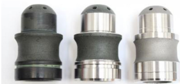
Fig. 9: Precombustion chamber—processing steps after laser welding (GE Jenbacher)
