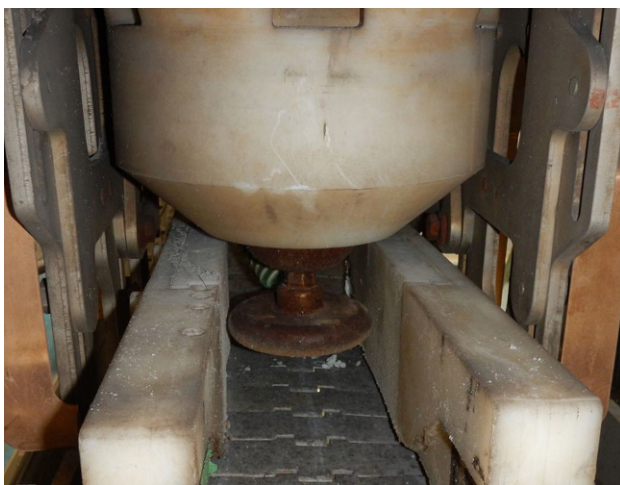
Fig. 3: Processing zone of the PWTS showing the pulse generator, the disk-shaped top electrode, the counter electrode (metal plate conveyor) and the insulation material for side guides
