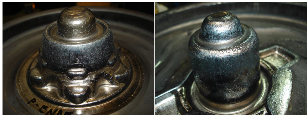
Fig. 2: Appearance of two closed-die forging dies after about 10,000 cycles [4]
