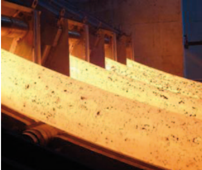
Fig. 1: Casting of 500-mm-diameter round blooms
