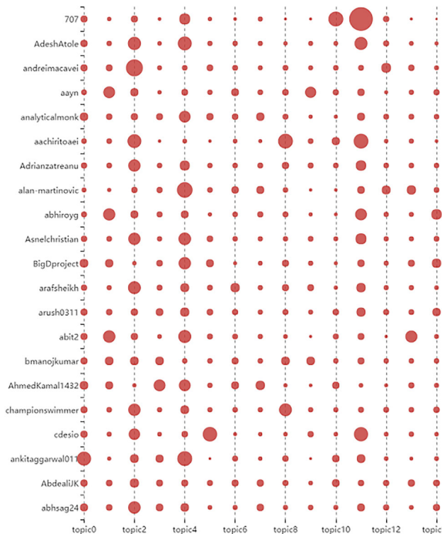
Fig. 6 Relation matrix of project coala visualized by punch card. The size of punch reflects the strength of the relationship between collaborators and topics. The larger the relationship value between collaborator and topic, the larger the corresponding node on the card
