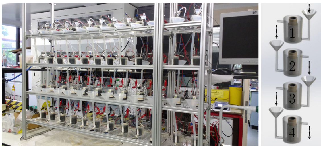
Fig. 5 Experimental setup. 12 cascades of 4 MFC units (left) and cascade schematic (right). Numbers show each MFC unit position within a stack and arrows indicate direction of feedstock flow. Five unique cascade designs and a control are evaluated in parallel, each duplicated for averaging
