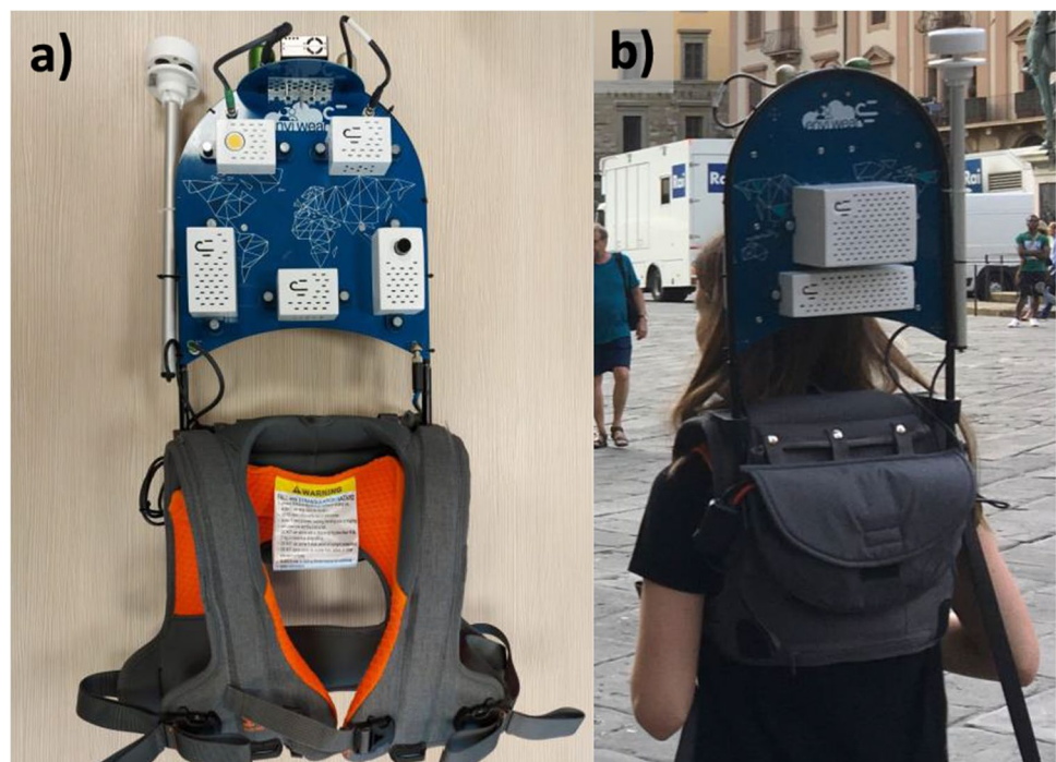
Fig. 2 The wearable equipment: (a) front view; (b) in use
