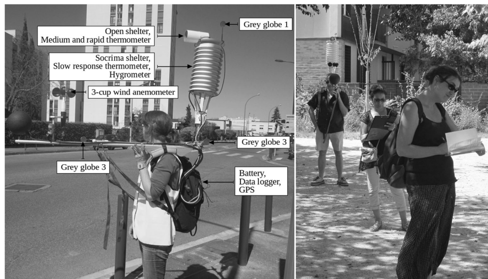
Fig. 2 Description of the portable structure for micrometeorological measurements (left) and photograph of the experimental protocol used during instrumented and commented walks (right)
