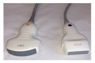
**Fig. 3** Convex and linear transducer. Left image: convex transducer with frequency of 3 to 5 MHz. They have a curved array that allows wider field of view. These are used for abdominal scans and have deeper penetration due to low frequency. Right image: linear transducers have a flat array and appearance. They have high frequency and are useful for small parts and shallow structures near the surface of the body. They produce a rectangular image with frequency ranging from 9 to 14 MHz
