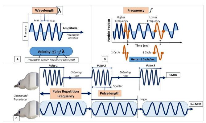
**Fig. 1** Physics behind ultrasound: basic physics concepts behind ultrasound imaging. **A**, **B** Depict the ultrasound wave as a sine wave. The wave travels through the tissue at a specified wavelength determined by the frequency (to which it is inversely related) at a specified amplitude. Frequency is the pitch, whereas amplitude is referred to as
