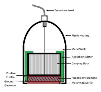
Fig. 4 Cross section of the transducer
