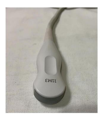
Fig. 2 Micro-convex array ultrasound transducer with frequency of 4 to  $10~\mathrm{MHz}$ , indicated for pediatric use as it has a small footprint
