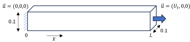
Fig. 23 3D clamped bar subjected to a horizontal displacement U_t at its right surface
