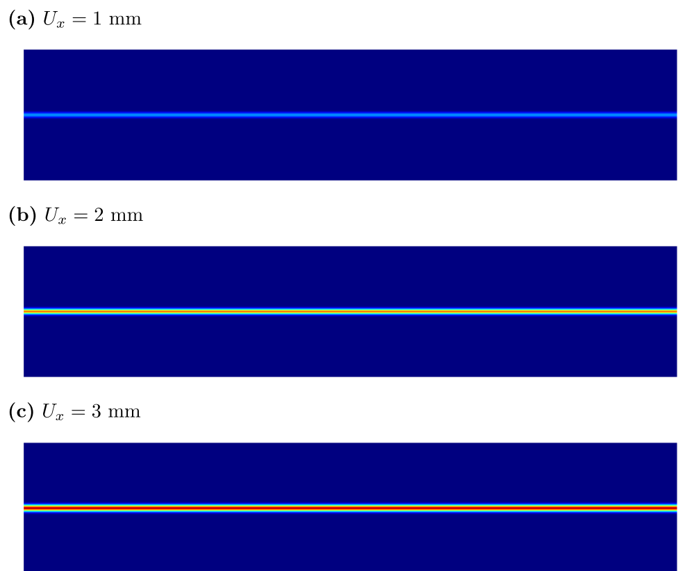
Fig. 5 The evolution of the phase-field variable at three time steps for the direct shear test. The imposed horizontal displacements, U_x , are: a 1 mm, b 2 mm, and c 3 mm
