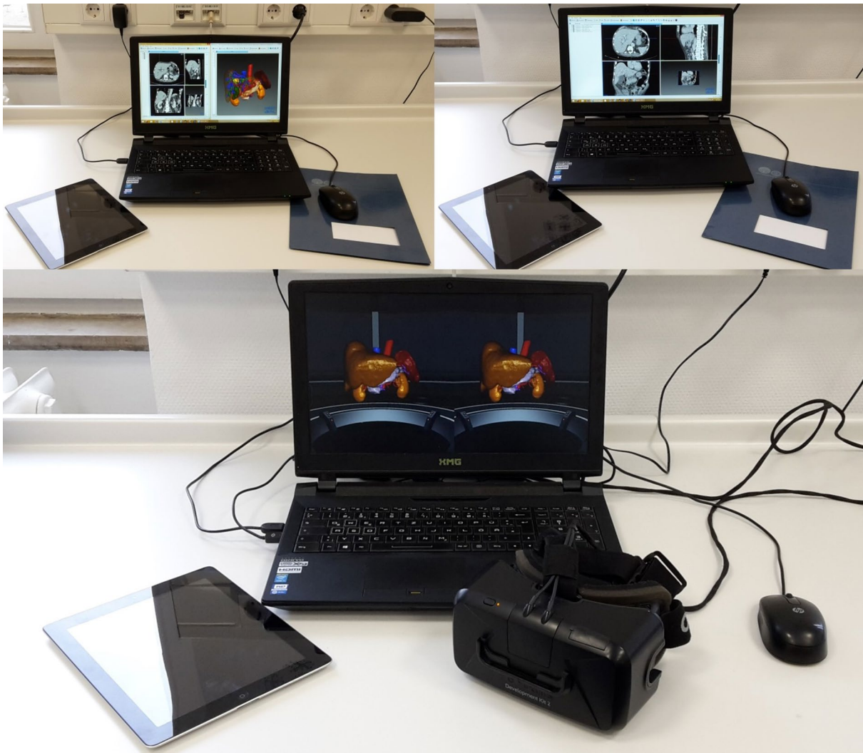
Fig. 4 Experimental setup for both 2D (top right), 3D (top left), and VR (below) evaluation (2D shown). The laptop and VR headset were used for case evaluation. The digital tablet was used for answering the questionnaire options
